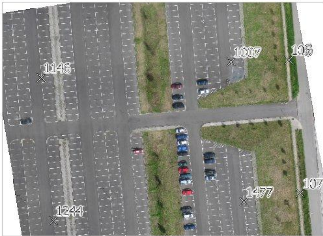
Testing area with reference point (left) and control points (right)
